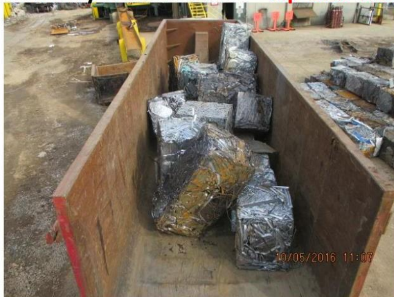
Unevenly loaded trailer – Tip over Risk
